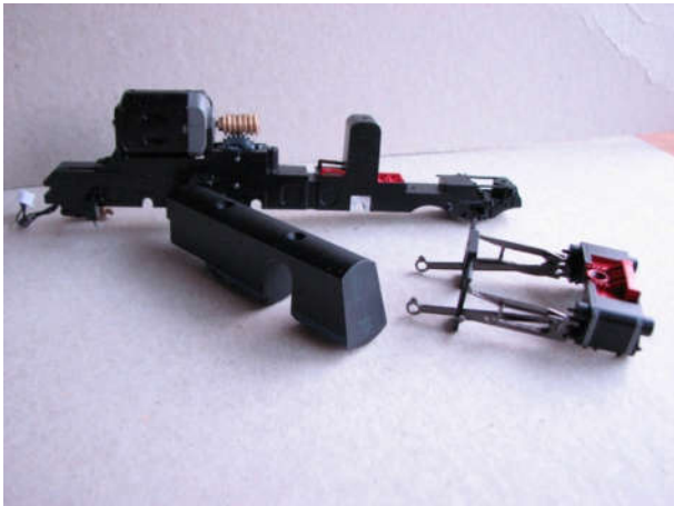
Cylinder assembly removal.
