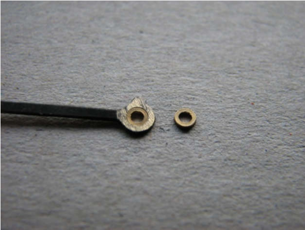
Bush in rod ready for soldering.
