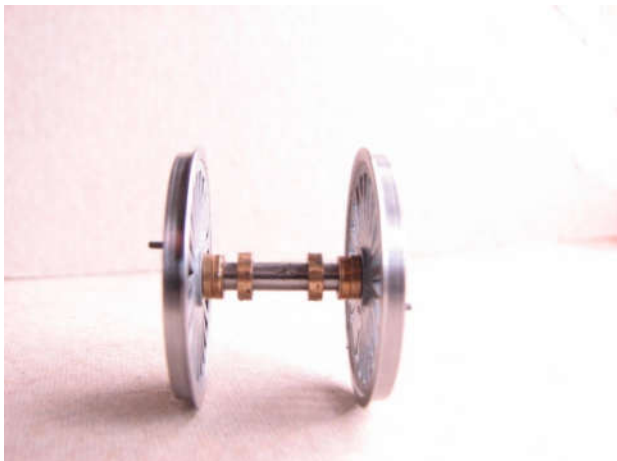
Rear wheels assembled – note spacing bushes.
