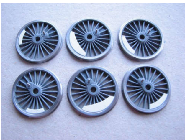
Gibson wheels fitted with crankpins.
