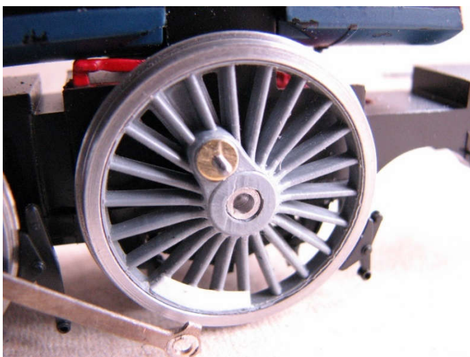
Romford washer in place.
